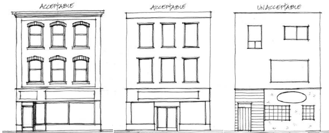
Figure 13: Alteration Examples - Storefronts
