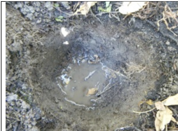
PLATE 7 TEST PIT FILLING WITH WATER
