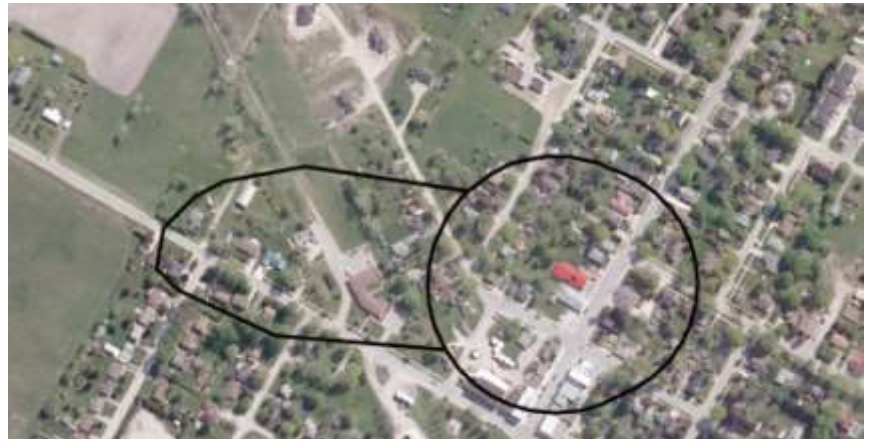
Example of a Wellhead Protection Area showing 100m circle and 2 year Time of Travel from a municipal well
